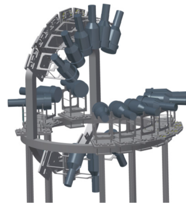
Figure 36: A schematic view of the half-meter flight-path detector array for measurements of neutron polarization asymmetries at HI \gamma S. Reprinted figure with permission from Ref. [158]. Copyright 2012 by the American Physical Society.
