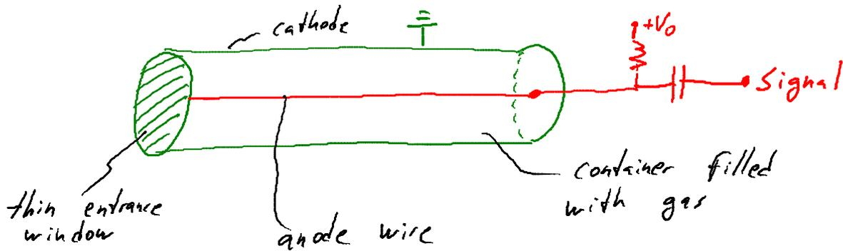
Radial electric field  $E = \frac{1}{r} \cdot \frac{V_0}{\ln(b/a)}$
